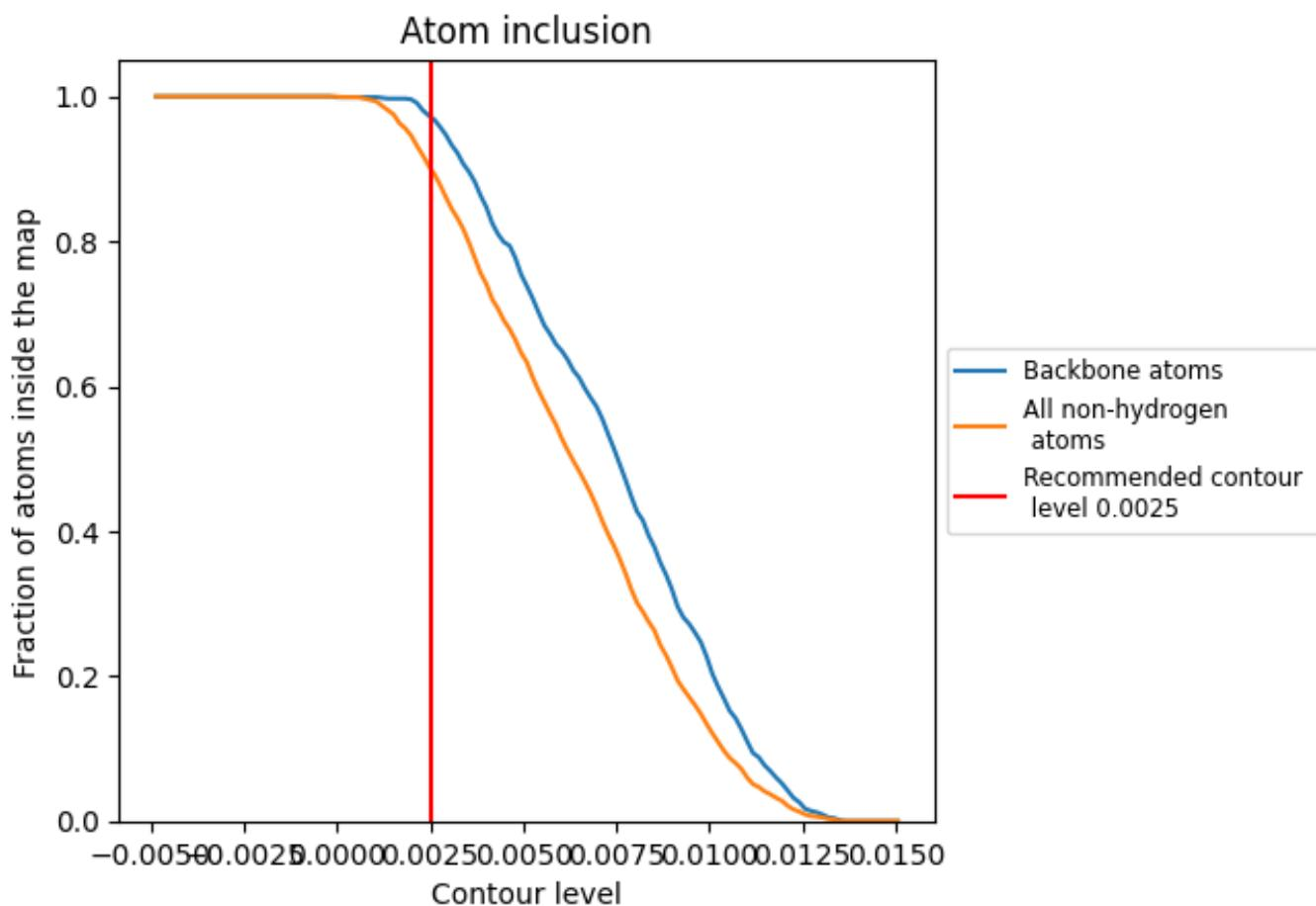
At the recommended contour level, 97% of all backbone atoms, 90% of all non-hydrogen atoms, are inside the map.
