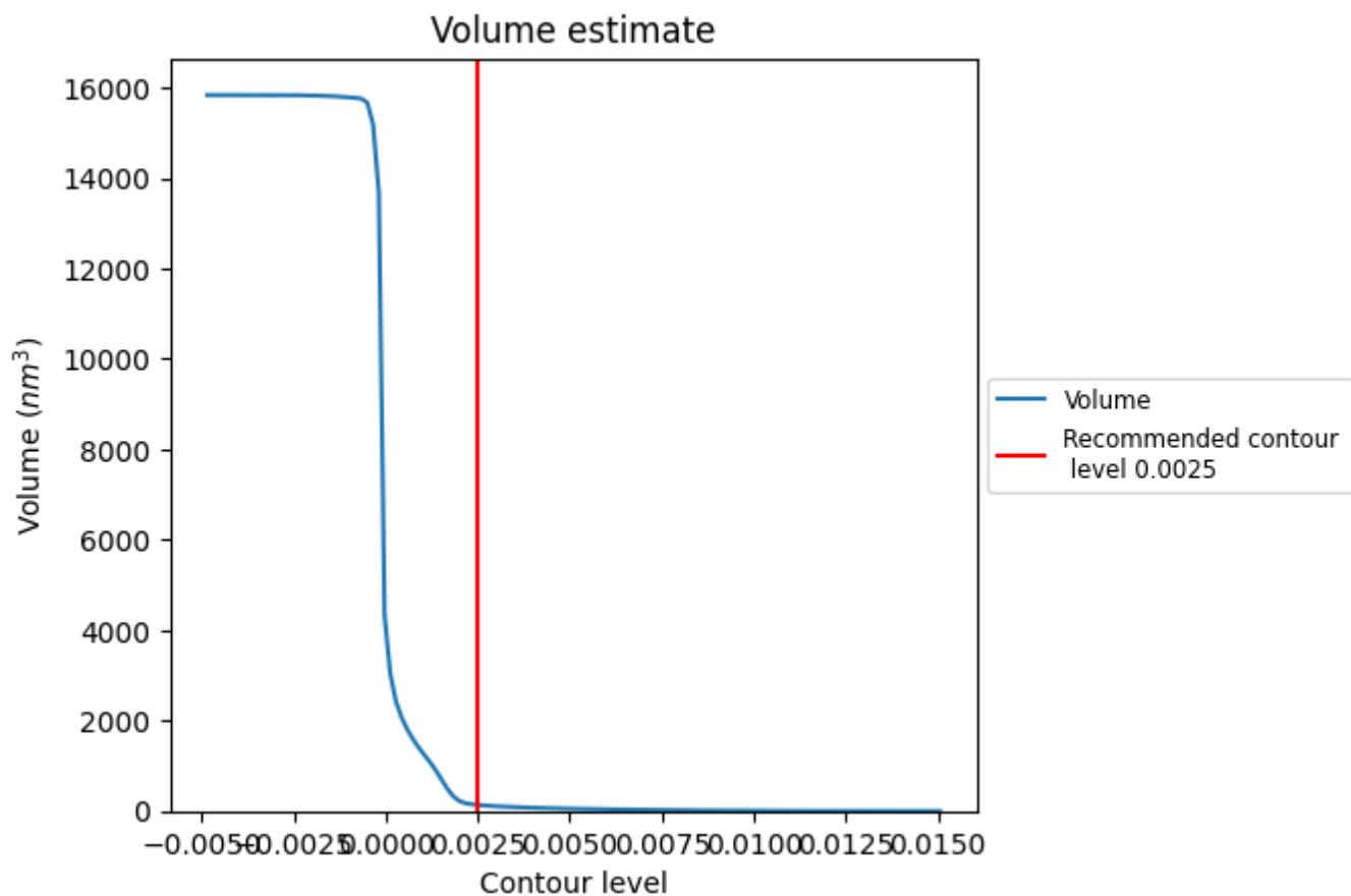
The volume at the recommended contour level is  $135 \text{ nm}^3$ ; this corresponds to an approximate mass of 122 kDa.
